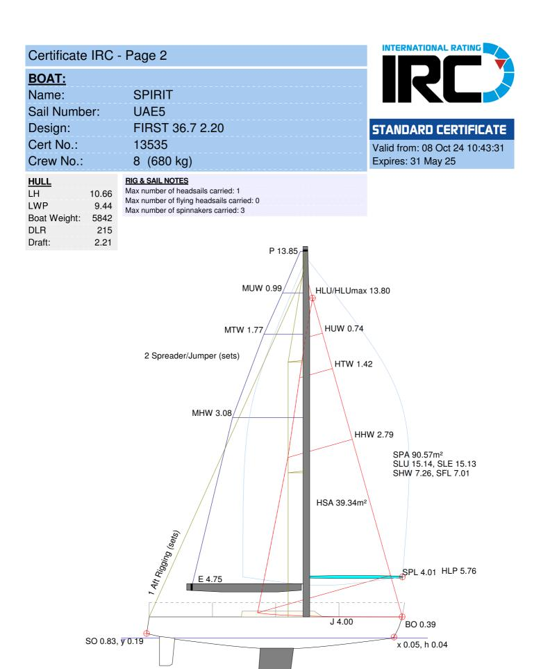
Units in metres unless otherwise stated. IRC Rule 13.3 The accuracy of the measurements supplied shall be the owner's responsibility. The boat drawing is approximated based on IRC rated data, if there is an error please contact your rule authority.
