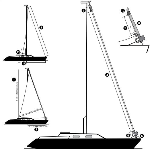
MEASURING TIPS. CHOOSE A CALM DAY IF POSSIBLE. STRETCH YOUR TAPE MEASURE AS TIGHT AS YOU CAN AND TAKE THE MEASUREMENT. IF NECESSARY MEASURE A FEW TIMES AND SEND US THE AVERAGE. DO NOT ALLOW FOR STRETCH, WE'LL DO THAT.
