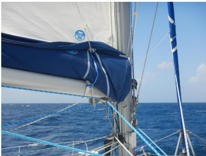
Here you can see how the stackpack is pulled closer to the sail
