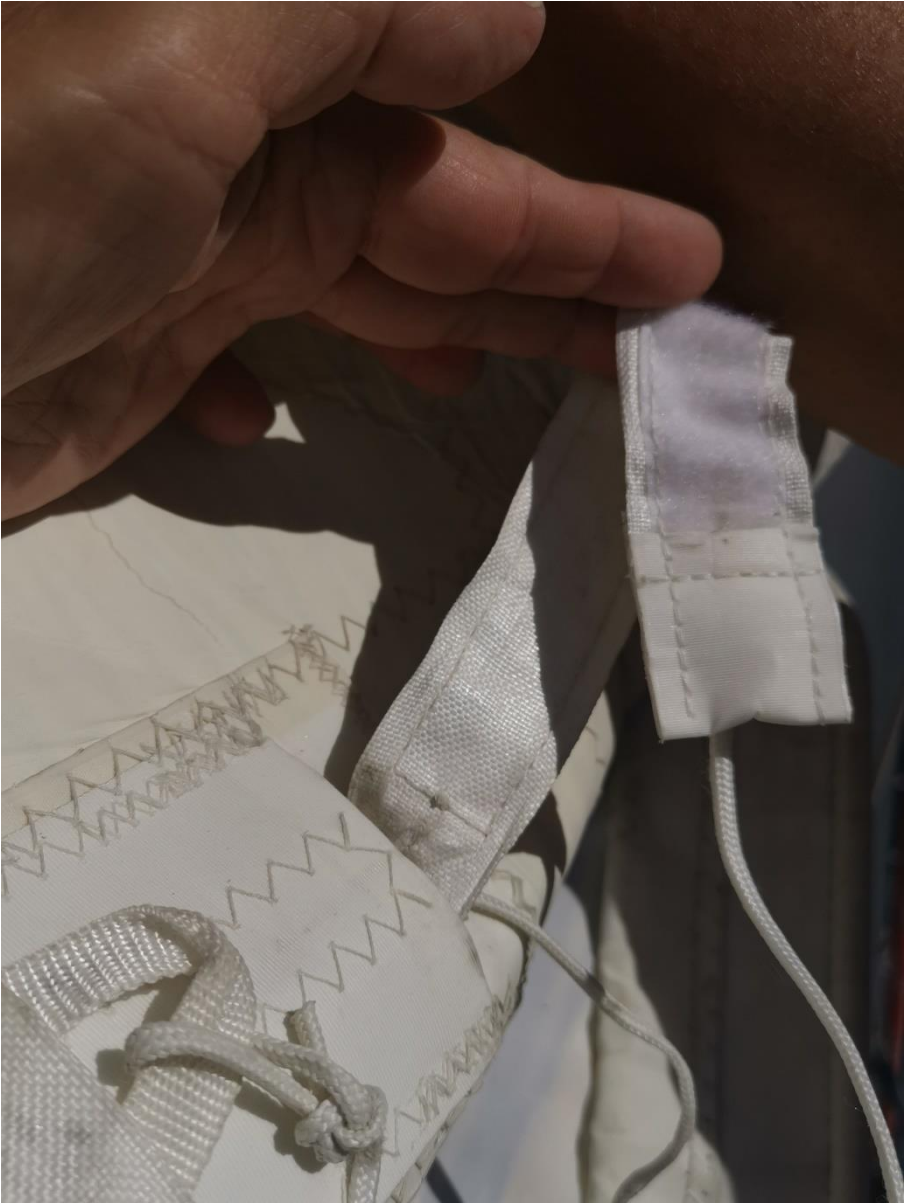
Batten pocket luff end batten nr 5 with velcro lock.
