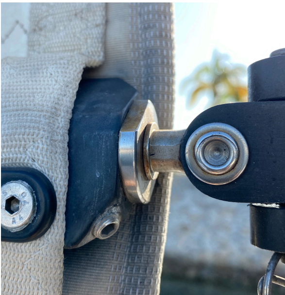
Luff Attachment at Full Batten Car
