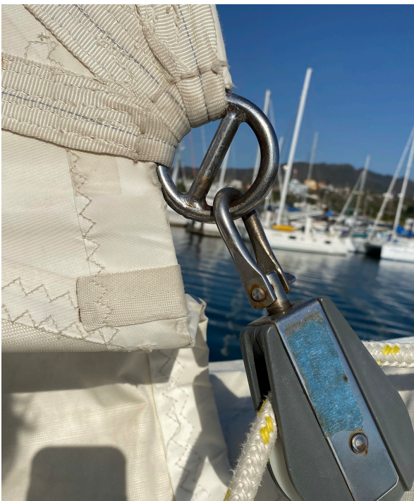
3rd Reef with pulley block
