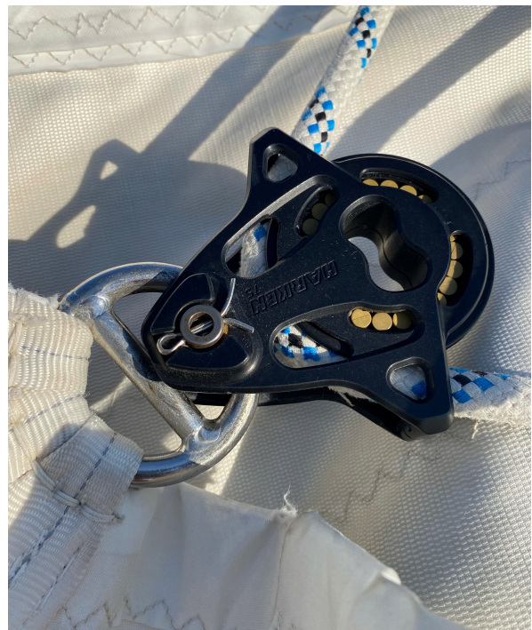
2nd Reef with pulley block
