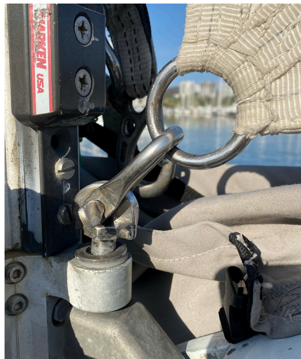
Mainsail Tack and Bottom of Track
