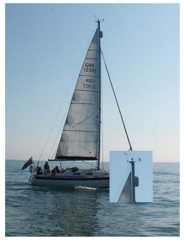
This a a picture of Buddle with its current main. The head of the sail is well below the black band and the luff measures 11.3 meters. The roach is well clear of the backstay and the boom clears the spray hood. Please note that the measuremnt of the main are not the same as that given on the internet. I understand that a shorter mast was fitted to some boats. The foot measurement is 3.9 meters.
