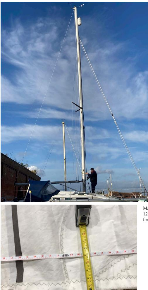
Mast bend was estimated to be 120mm on the mast and confirmed on the sail.
