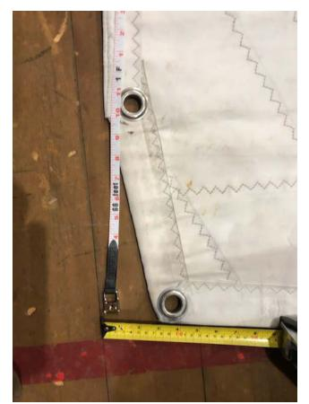
The sail was off the boat but I measured on the boat without the sail and checked once I had got the sail back from the sailmaker. I found the cut back A to be 92mm and the cut up B 7mm.
