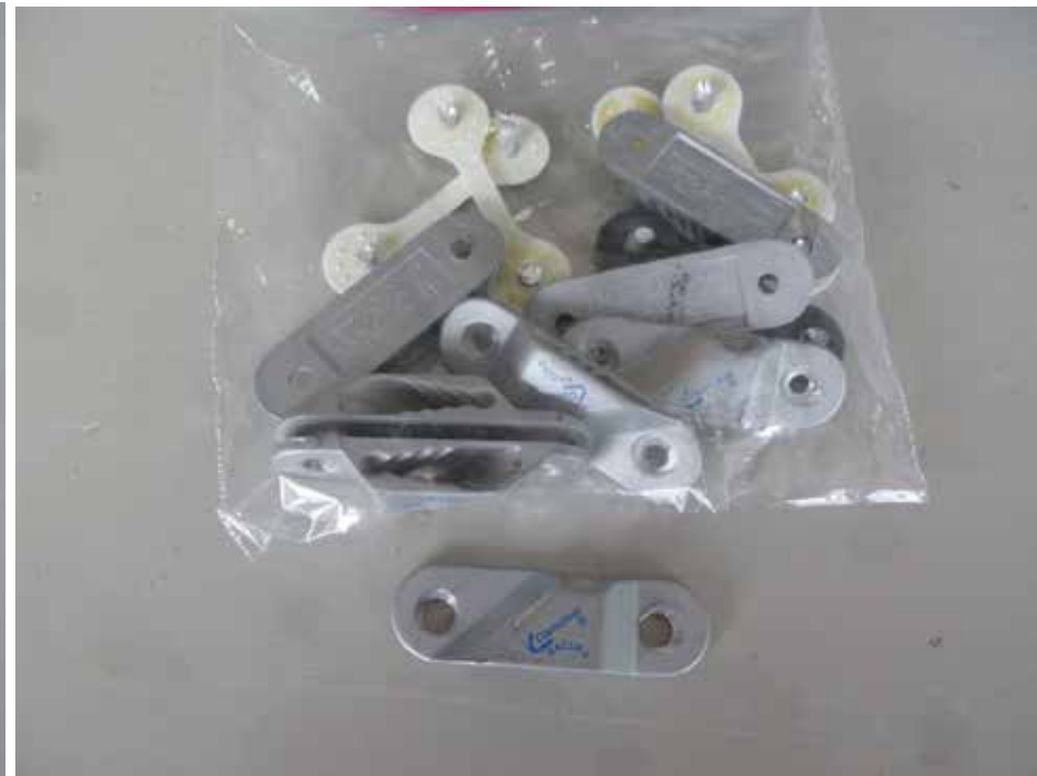
Cleats for leech line, needed just above each reef point at luff and leech. Some of these were riveted in place, some were hand stitched. Your choice.
